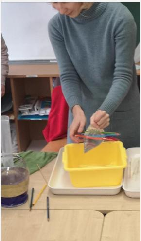
Take two plastic glasses. Make holes around on at the same level in one of the glasses and make vertical line of holes in the other glass. Close holes with scotch from outside. Pour water into the glasses and take scotch off. What is happening? We have the same streams of water from the holes around the glass, but different streams from holes arranged vertically. The hughest stream is weakest and the bottom one is the strongest. Why?
