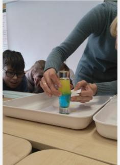
Take two small glasses and fill them with cold and warm water. Put different colors into them. Cover warm water glas wiht peace of paper. Overturn it and put on a cold water glass. Take peace of paper out carefully and let water to mix. But it is not mixing - different colors stay in their glasses – just small area is mixing. Why?
